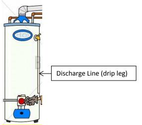
**29-5-15** <u>Water heaters installed in garages.</u> Water heaters having an *ignition source* shall be elevated such that the source of ignition is not less than 18 inches (457 mm) above the garage floor. (IRC P2801.6)
